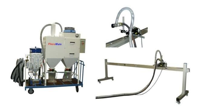
All used media and contamination is being sucked out of the cabinet or away from the roll by the ventilator or vacuum source and separated from the air stream by the pre-separator cyclone and filter unit.
